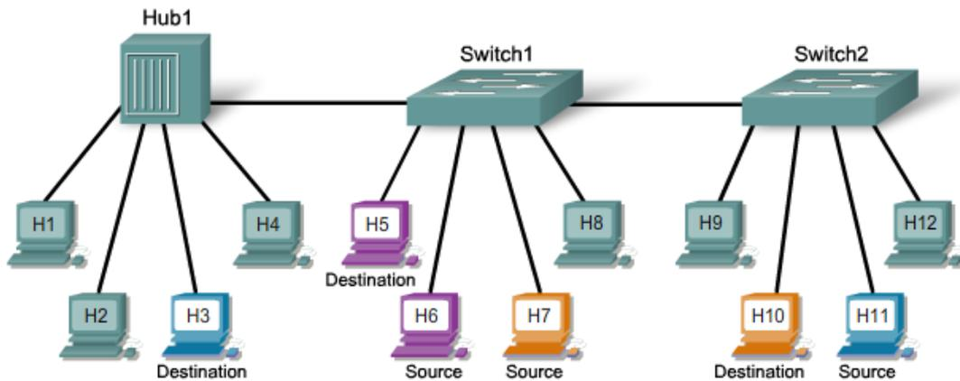
If Host9 sends a message to Host6, and the destination MAC address is in the MAC table for both switch1 and switch2, which host devices will receive the message?
